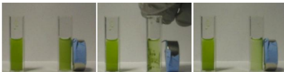
Figure 3. Movie stills captured during the adsorption of Dunaliella salina by AP-Fe 3 O 4 -MSN. Left cuvette is the control and the right cuvette shows the algae accumulation using an external magnet.
